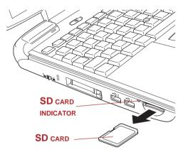
Figure 8-6 Removing an SD card
